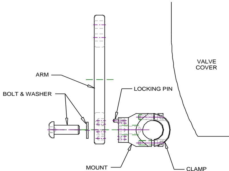
Notice that if you hold the mount and clamp together there is a gap only on one side. This gap should be towards the rear of the engine guards or facing you as you sit on the bike.
